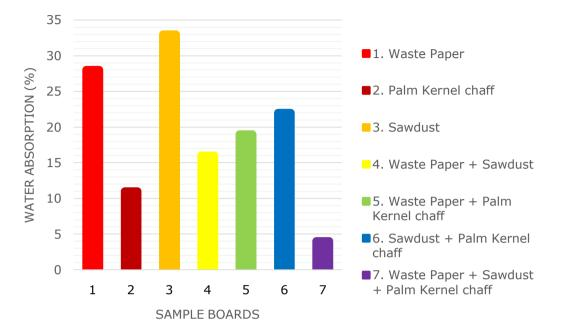
Figure 1: Water Absorption Percentage of Sample Boards
