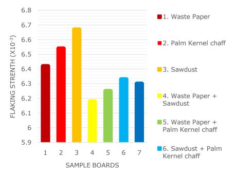
Figure 2: Flaking Test of the Boards
