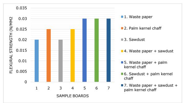
Figure 3: Flexural Strength Test
