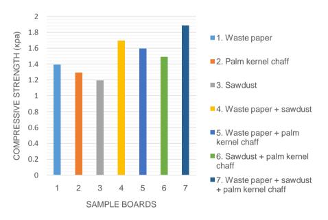
Figure 4: compressive Strength Test
